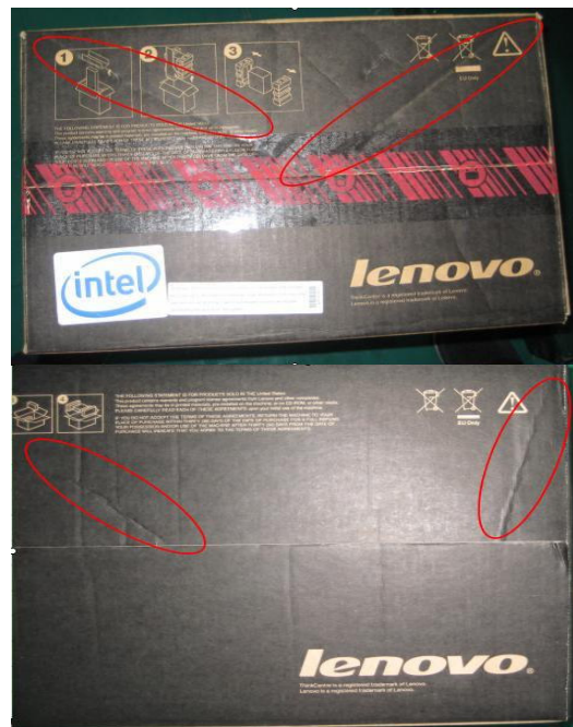
Picture2: Wrinkle formed by Outside force
