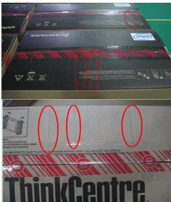
Picture 1: Wrinkle along corrugated flute direction
