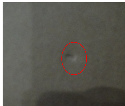
Picture10: Punctures not through and diameter less than 2cm
